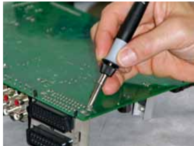
High-mass through-hole soldering with the i-TOOL
