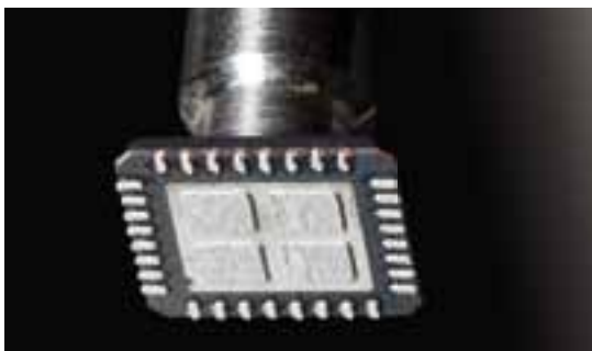
MLF 32 with solder paste printed on the bottom
