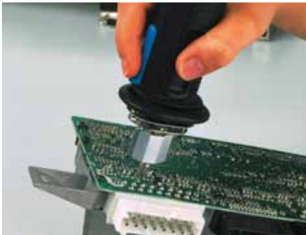
High-mass through-hole desoldering
